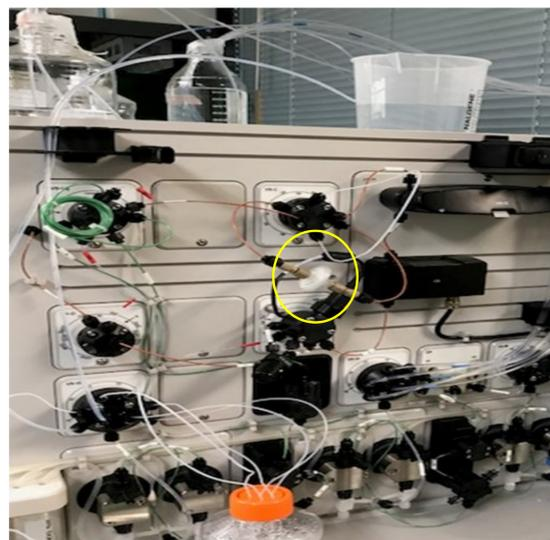
Figure 2: Virosart Max Installed on AKTA Avant
